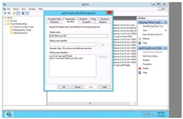
Figure 5-6 Adding File Plan Builder Site URL to Relying Identifier List
