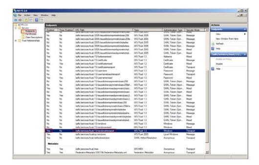
Figure 5-5 Enabling WS-Trust
